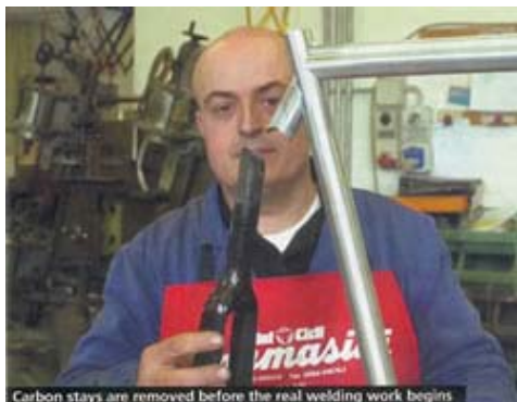
Carbon stays are removed before the real welding work begins
