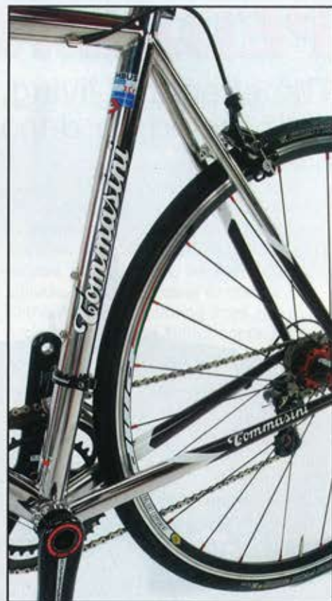
The welded X-Fire provides a noticeably stiffer ride than found on the lugged Tecno. You've got to love the polished tubes.
