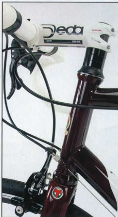
The X-Fire gives a nod to modernity not just with its stainless steel tubes, but also a carbon fork and 1 1/8" steerer.
